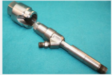
50D018 Adaptor Mercedes To Be Used With Impact Hammer
